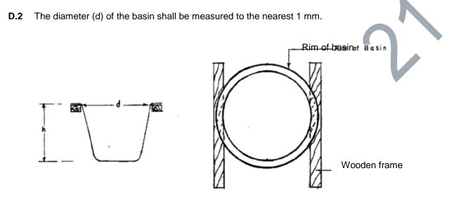
Figure D.1 — Distortion test
